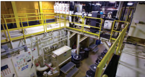
Twin STAR Vacuum filters deliver "super" clean coolant at a constant temperature to more than 20 machining centers.
