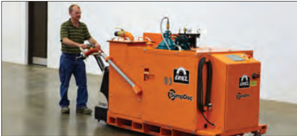
The new SumpDoc provides complete solids removal and fluid recycling at the sump.
